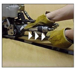
Note: Before continuing, make sure the TOP STRAP and the seal is still in position, as described above. Note that the BOTTOM STRAP will be positioned in the channel on the bottom surface of the breaker foot. This too, is necessary to maintain strap alignment during tensioning.
