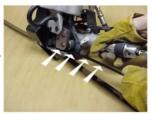
2. Push the tool forward until the seal-stop contacts the end of the seal.
