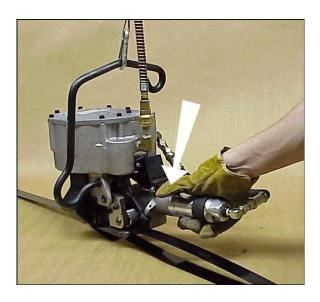
4. If strap alignment is unsatisfactory and it becomes necessary to shut off the tool during the tensioning portion of the cycle, push down on the stop lever.
